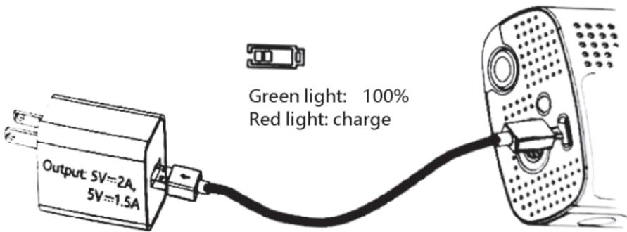
The USB charger is recommended to use 5V /1A. Use the Micro USB charging cable to connect the air pump and power adapter (sold separately) for charging.
